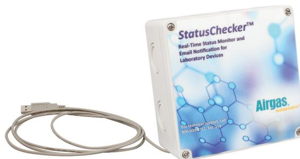
The StatusChecker can also be used to monitor any contact switch, such as a cryogenic freezer door. The StatusChecker can notify you whenever the door is opened and provide a log of every time the event occurs.
