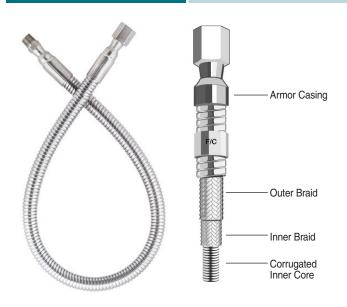
**Description:** These flexible metal hoses are fabricated from 316L stainless steel corrugated bellows and feature an inner core reinforced with two stainless steel braids. The inner core and double braids are welded to the end fittings and a protective armor casing is attached to the exterior. These hoses are ideal for high-pressure and low-pressure plumbing connections. With the additions of CGA connectors, they make very usable flexible pigtails.
