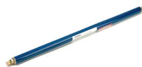
changes may introduce moisture. The trap consists of a 24" metal tube filled with ½ pound of molecular sieve 5A and is capable of reducing water concentration to less than 0.1 ppm.
